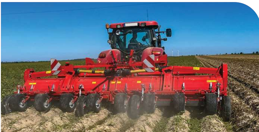
The Toppa 800 with ridge pressure wheels called 'RidgeRunner' in working position.
