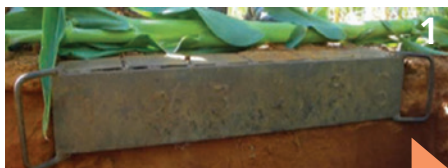
1 A steel plate used to take soil samples. (Source: Jan du Toit, agricultural advisor, Omnia)
