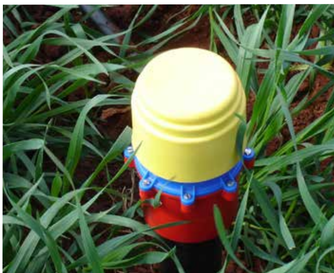
Figure 4: Capacitance probe with sensors at different depths (e.g. every 10 cm). The instrument is lowered down the soil profile through an access tube.
