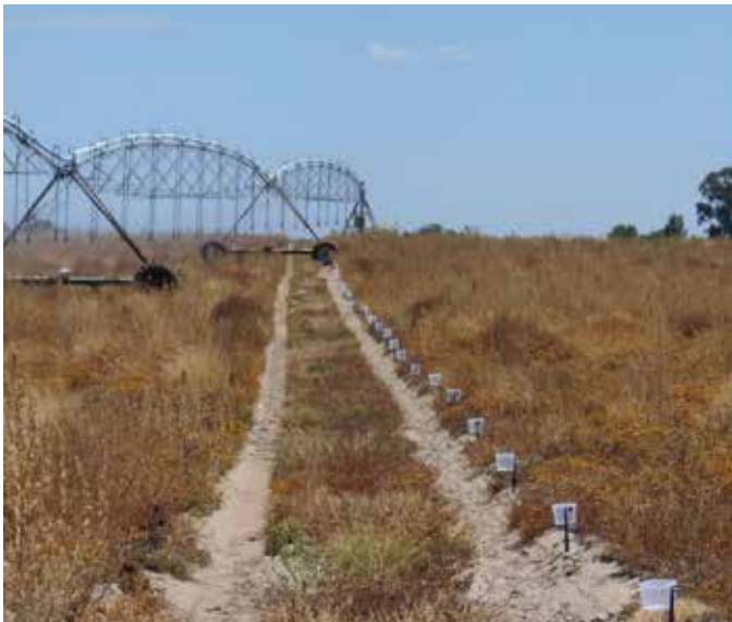
Figure 7: Rain gauges are used to evaluate the distribution uniformity of a centre pivot irrigation system
