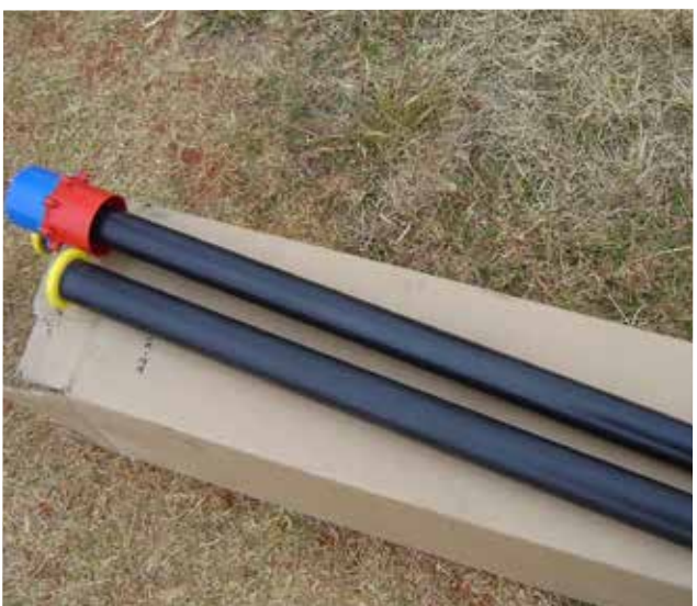
Figure 4: Capacitance probe with sensors at different depths (e.g. every 10 cm). The instrument is lowered down the soil profile through an access tube.
