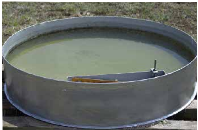
Figure 1: In the past Class A pan evaporation (Epan) was commonly used as estimation of atmospheric evaporative demand and used together with crop factors to calculate crop water usage (ET).
