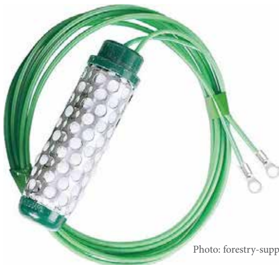
Figure 2: Watermark® electrical resistance sensor (left) and digital gauge (right) for measuring soil water potential.
