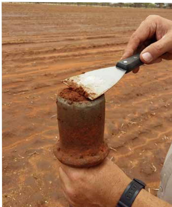
Figure 1: Sampler with known volume for the collection of soil samples
