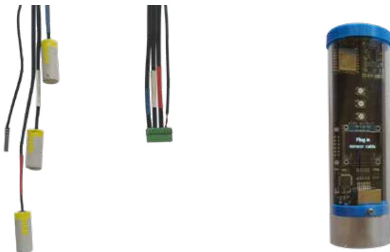
Figure 3: A set of Chameleon sensors for measuring soil temperature at one depth and matrix potential at three different soil depths (left); and LED reader (right).
