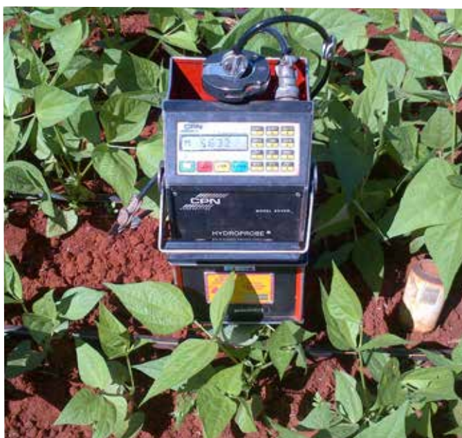
Figure 2: The neutron probe is placed on top of an access tube and the radioactive source is lowered down the access tube to measure water content of the different soil layers.
