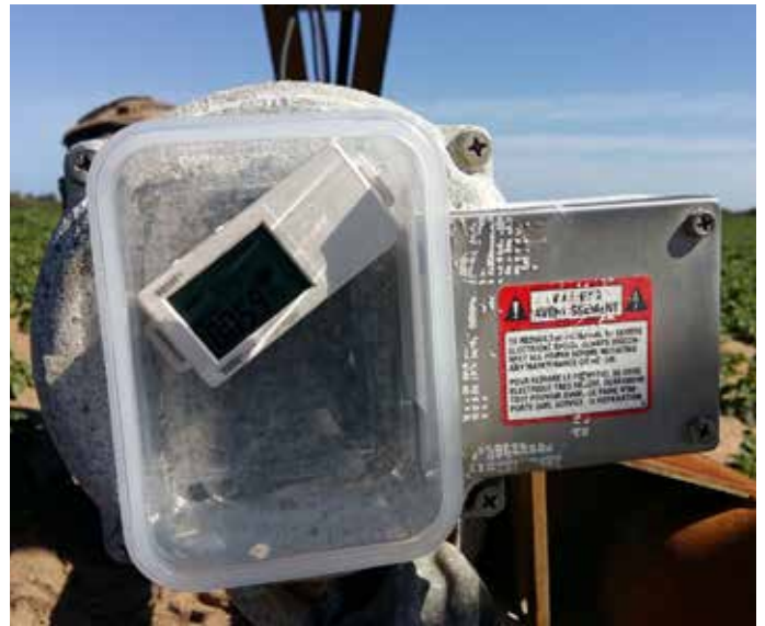
Figure 8: Mounting of an electromagnetic sensor to monitor pivot run time
