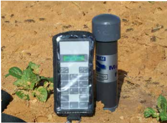
Figure 5: Example of a capacitance probe that is installed directly into the soil. It has sensors at five different depths (every 10 cm) and data can be downloaded with a radio logger (left on the photo).
