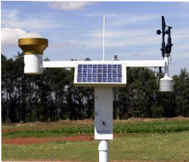
Figure 3: Example of an automatic weather station for the collection of prevailing weather variables that can be used to calculate atmospheric evaporative demand (ET o ).
