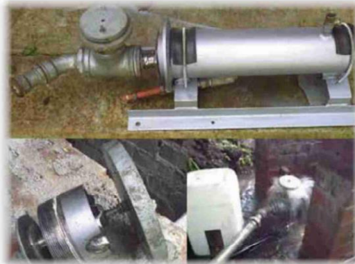
Fig. 1: Assembled ram pump. Initially the impulse valve (bottom left) was fitted with disk-weights which were removed later as it operated better without them. Operation after installation shown bottom right.
