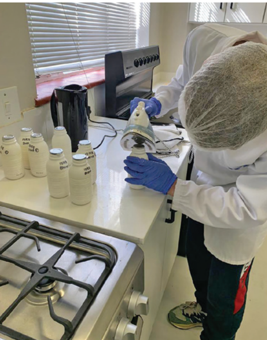
The potato milk is bottled, sealed, and taken to a facility for in-pack retort sterilisation.
